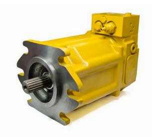
Our MHPR series pumps come equipped with a load sensing and pressure cut-off control. The load sensing regulator adjusts the amount of flow from the pump to maintain a given pressure differential through a throttling device. Essentially, this matches system flow and pressure by destroking the pump and consequently saves fuel and reduces heat generation.
